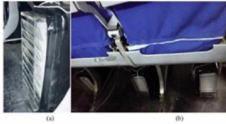
Fig. 5. (a) A close-up view of a diffuser and (b) the diffusers installed under the seats.
